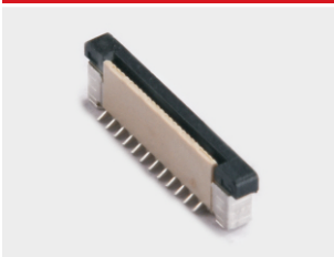
CONN FFC 1.00mm,Anti-needle, SMD,Vertical,with ZIF
