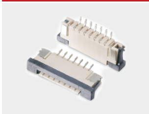
CONN FFC 1.25mm SMD, Lower Contact , with ZIF
