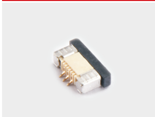
CONN FFC 0.50mm,SMD,Horizontal, Upper Contact , with ZIF
