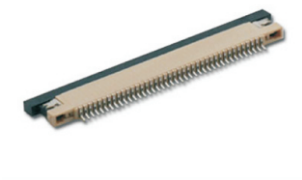
CONN FFC 1.00mm,SMD,Horizontal, Upper Contact ,with ZIF
