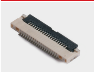
CONN FFC 0.50mm,SMD,Horizontal, Lower Contact , with ZIF
